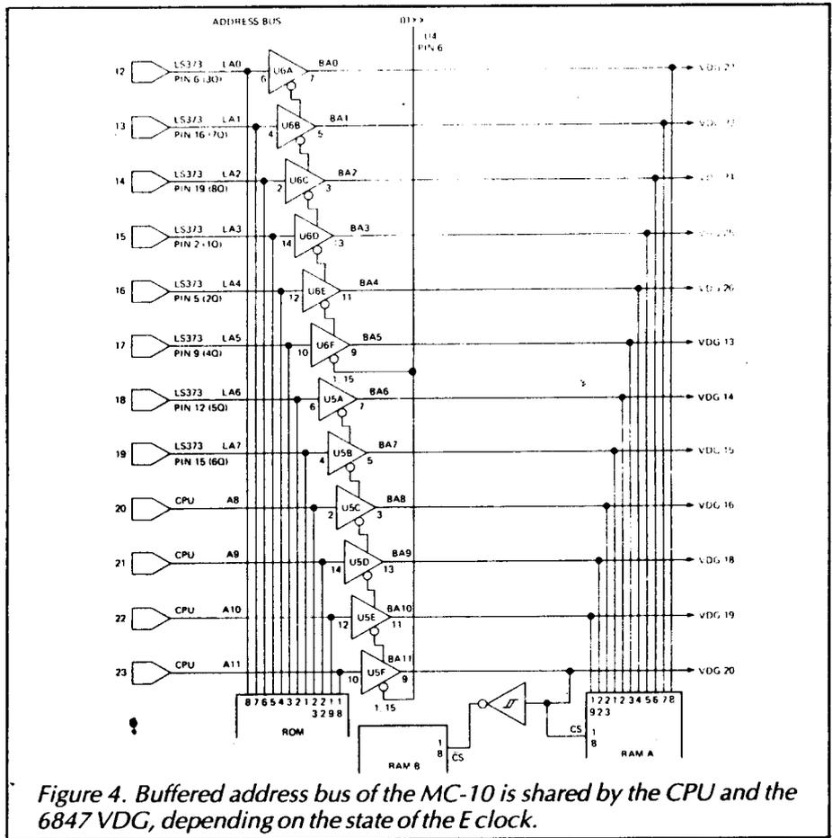
Figure 4. Buffered address bus of the MC-10 is shared by the CPU and the 6847 VDG, depending on the state of the E clock.
