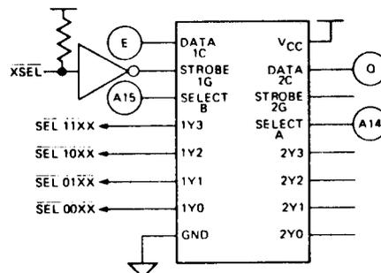
Figure 1. On-board memory decoding of the MC-10, before the Radio Shack correction.
