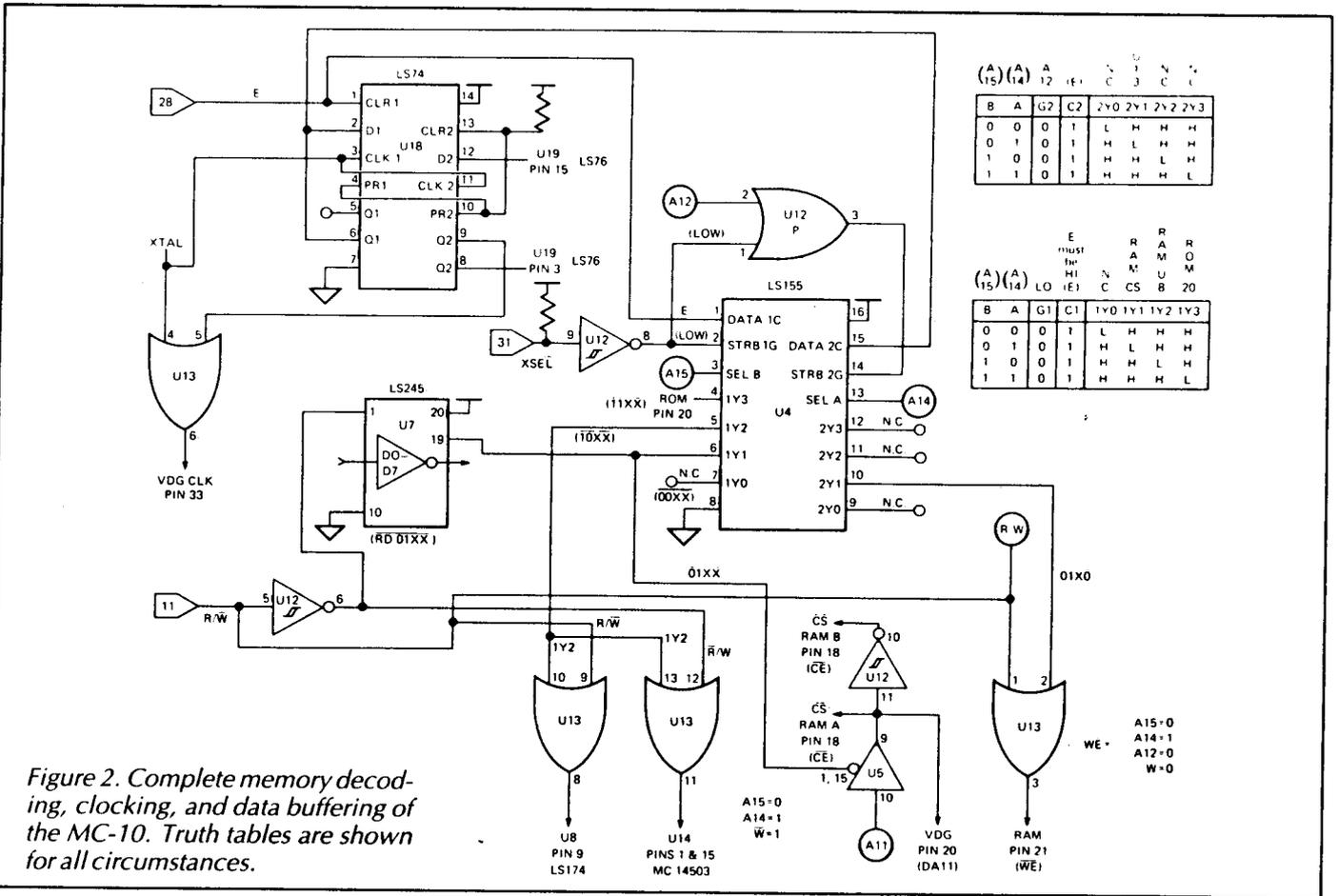
Figure 2. Complete memory decoding, clocking, and data buffering of the MC-10. Truth tables are shown for all circumstances.
