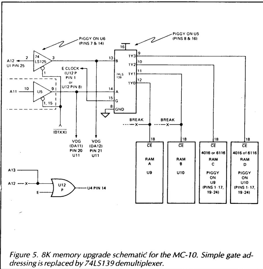
Figure 5. 8K memory upgrade schematic for the MC-10. Simple gate addressing is replaced by 74LS139 demultiplexer.
